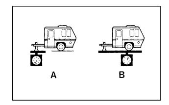
If you're using a weight-carrying hitch or a weight-distributing hitch, the trailer tongue (A) should weigh 10-15 percent of the total loaded trailer weight (B).
